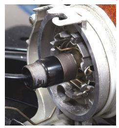
After the sealing cap is installed, you can store the bulb barrel ramp tool over the bulb-to-driver-module connector so it's easily available next time the sealing cap needs to be removed and reinstalled.
