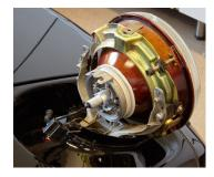
Tilt the cap so the bottom of cap is closest to the headlight assembly as shown and feed LED H4 bulb's wire through the center hole.
